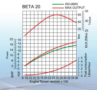
Based on theoretical propeller loading - matched at full speed
